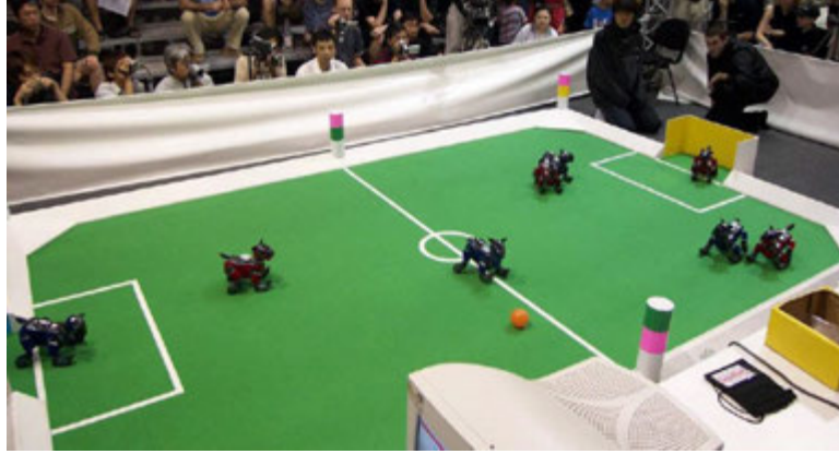
Figure 4.7: AIBO robots on the RoboCup soccer competition. Note the engineered landmarks positioned at the corners and the middle of the soccer field. AIBO being a relatively small robot, its limitations on computational resources requires both conspicuous and unique landmarks. The field is tracked by color via a small optical sensor under the robot, and the ball by color. In the original robot kit developed by SONY, AIBO comes with a plastic bone and a ball to play with. Both items are colored neon-pink such that they would not possibly blend in with the furniture in a typical home, so they could attract the sensors of AIBO under any circumstances.
