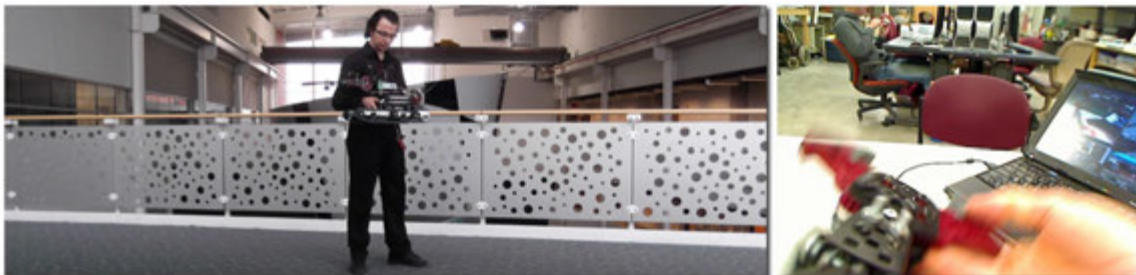
Figure 3.69: Left: Intended to be human portable Virgil-II weighs only 10 kilograms while providing sufficient torque to penetrate 15mm plywood. Right: Live high definition video stream from Virgil claw. This stream serves both machine vision and surveillance purposes.
