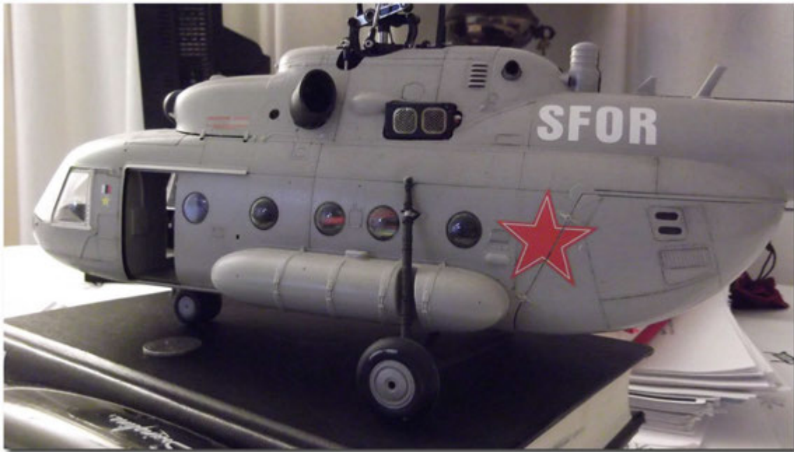
Figure 3.103: The sliding door is functional, and removable. The cockpit is authentic to the aircraft. Fuel cells are loaded through this door, as well as the cargo doors. Just like the real-life counterpart, my MI8 features driven tail and can capably autorotate. This is the smallest aircraft so far to benefit from VINAR.
