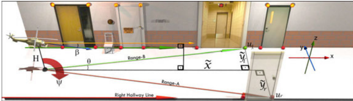
Figure 2.47: A three dimensional representation of the corridor with respect to the MAV. Note that the width of the hallway is not provided to the algorithm and the MAV does not have any sensors that can detect walls.
