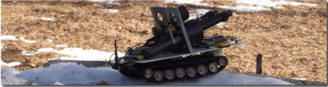
Figure 3.65: \mu Virgil Mobile UAV Launcher. This semi-autonomous MAV carrier deployment vehicle carries a pneumatic catapult designed to launch a small aircraft at high speed. It is more fuel efficient than most flying vehicles which makes it an ideal choice to bring the UAV as close as possible to mission site. It further allows take-off in virtually any environment, because it can negotiate a very wide variety of rough terrain.
