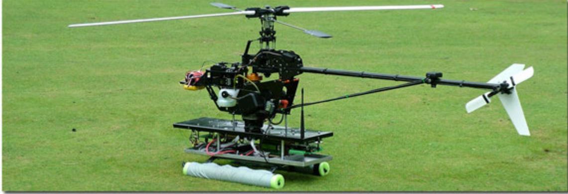
Figure 3.58: The \mu CART aircraft before a mission, at full payload, standing by for fueling. Engine starting and refueling are about the only manual operations for this machine.
