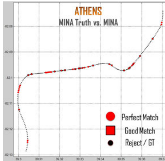
Figure 7.90: MINA detections during simulated AFRL flight over Athens; compare to Figure 7.89. A small dot indicates ground truth as well as dead reckoning. A square indicates a match with high certainty. A large dot indicates a match with medium certainty. There is some evident clustering of matches, which indicates they have been matched across multiple frames.
