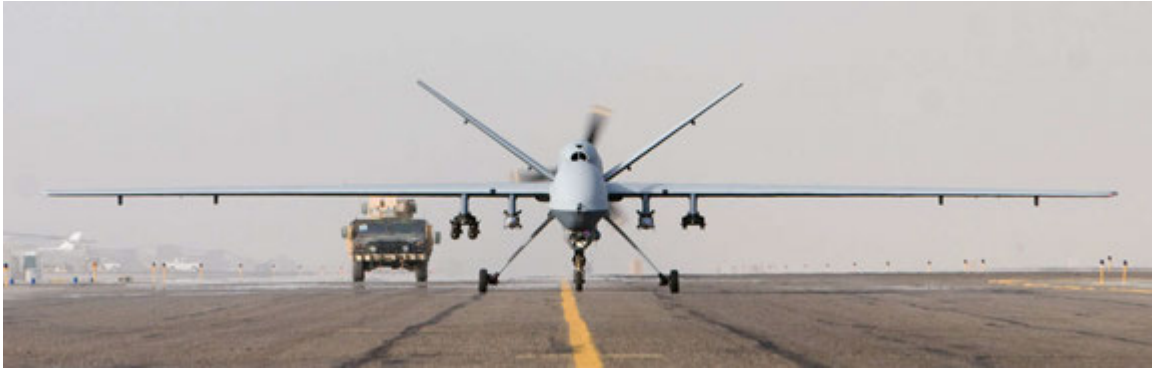
Figure 1.7: The Reaper UAV. Despite popular belief, this is a remote controlled aircraft and not a robot.
