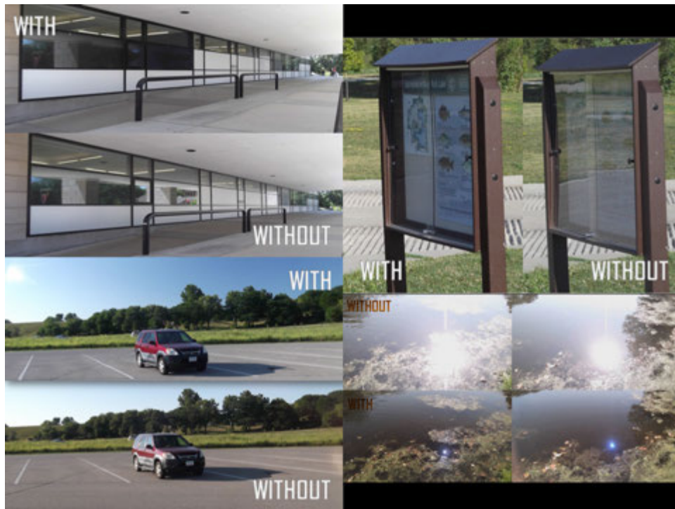
Figure 7.84: Polarizing filter in front of the lens removing adverse effects of glare.
