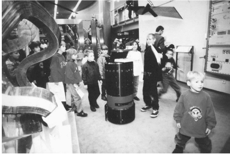
Figure 4.6: The Rhino robot in the Deutsches Museum Bonn. Note the sheer size of Rhino. This type of robot is easy to build, it can carry very powerful computers and high quality sensors (and quite a wide array of them) on board to make the task of an EKF engine easier.
