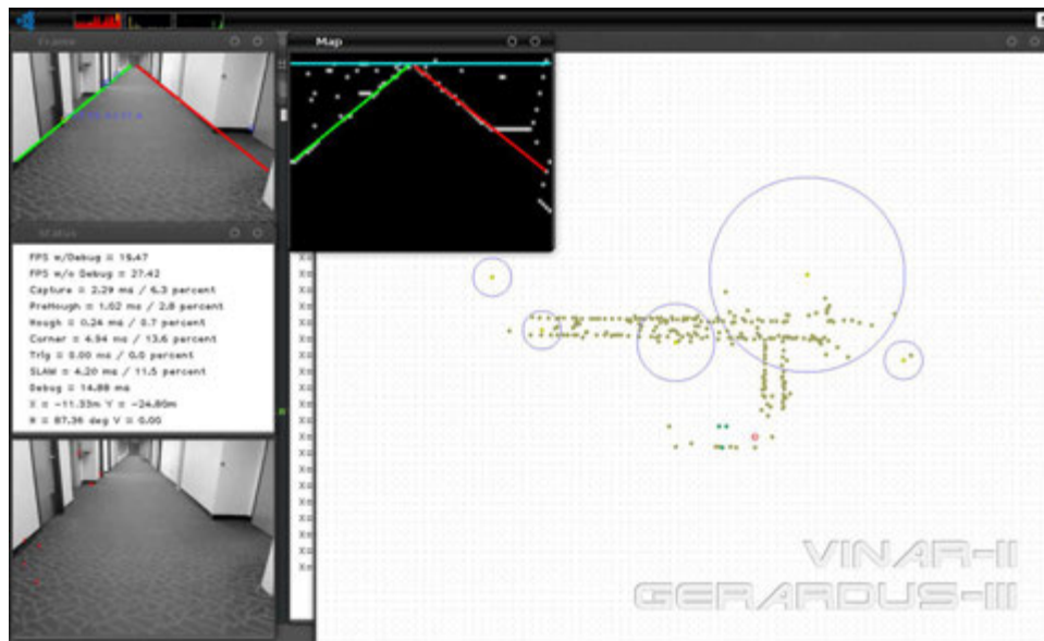
Figure 2.49: Graphical User Interface of VINAR-II with GERARDUS-II Mapping Engine. This is also an actual screenshot of the Saint Vertigo Helicopter during flight, as it appears at a ground station.
