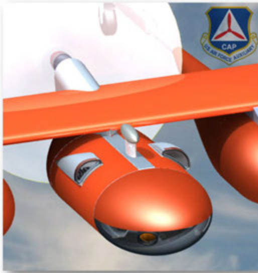
Figure 3.90: Aircraft VINAR hardware is blended into the fuselage without requiring use of an external turret, providing improved aerodynamic efficiency.
