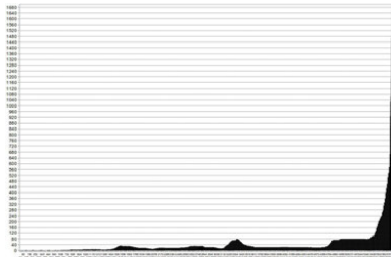
Figure 6.23: Example-1 positioning error propagation in time. Vertical scale is in m^2 and horizontal scale in state observer motion steps.
