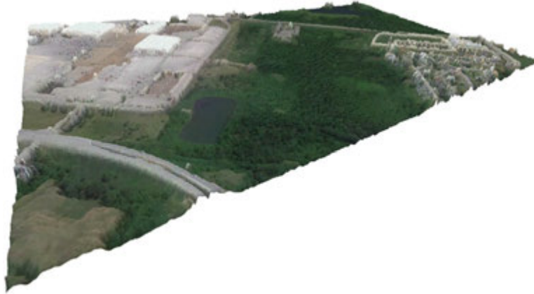
Figure 7.59: After successful wavelet decomposition, the spectral layers can be rendered in a meshgrid as different heights with respect to frequency band, resulting in an image where objects of interest are embossed, such as roads and parking lots shown here on a curve of Interstate 35.
