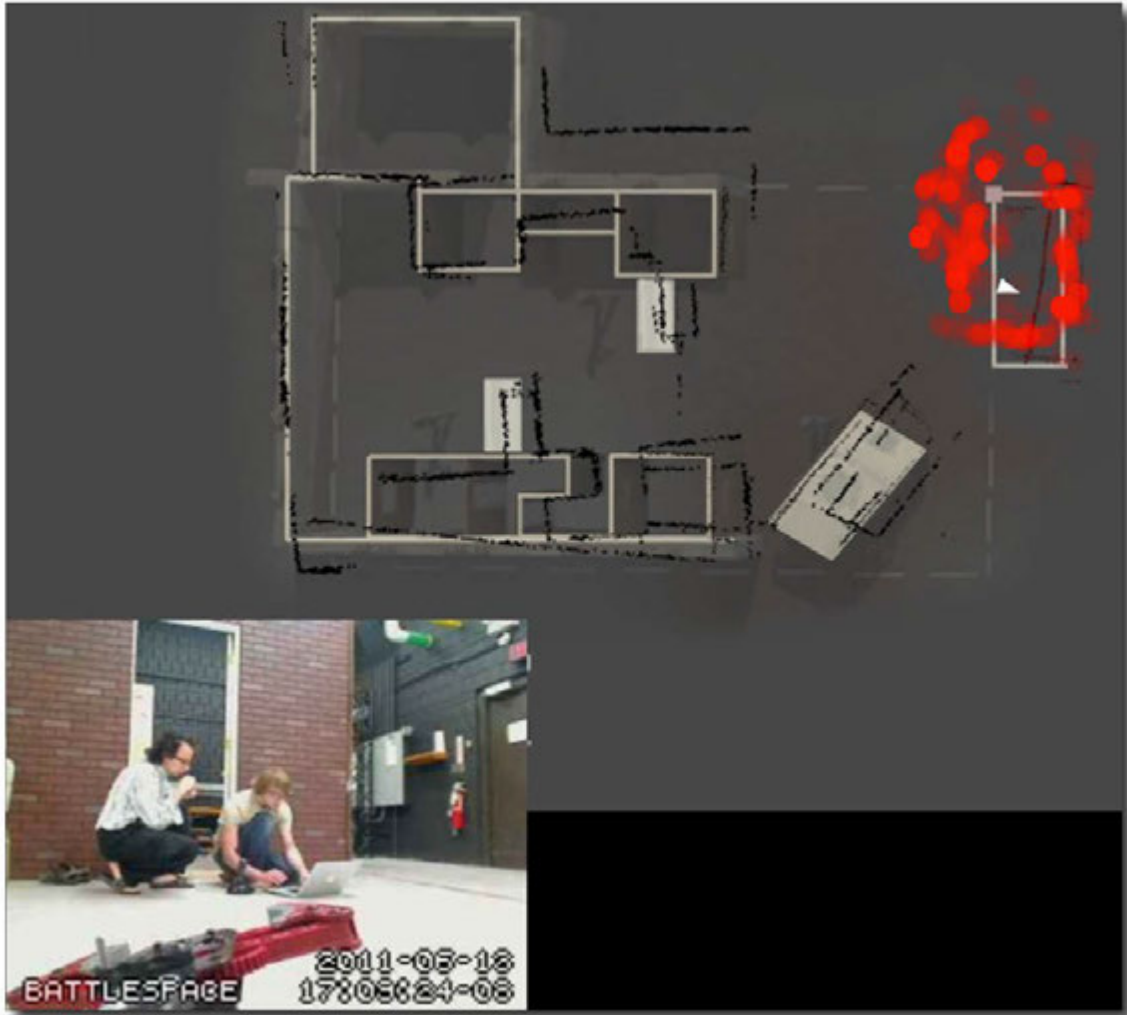
Figure 8.23: VINAR map and threat map (Americium traces, shown in red) of the environment by Virgil. In the red area there is an IED planted, while the robot was not looking. The robot scouts around the base and had a matured understanding of the base map, where introduction of new objects and senses are considered threats and flagged accordingly. This information is propagated to all Battlespace units.
