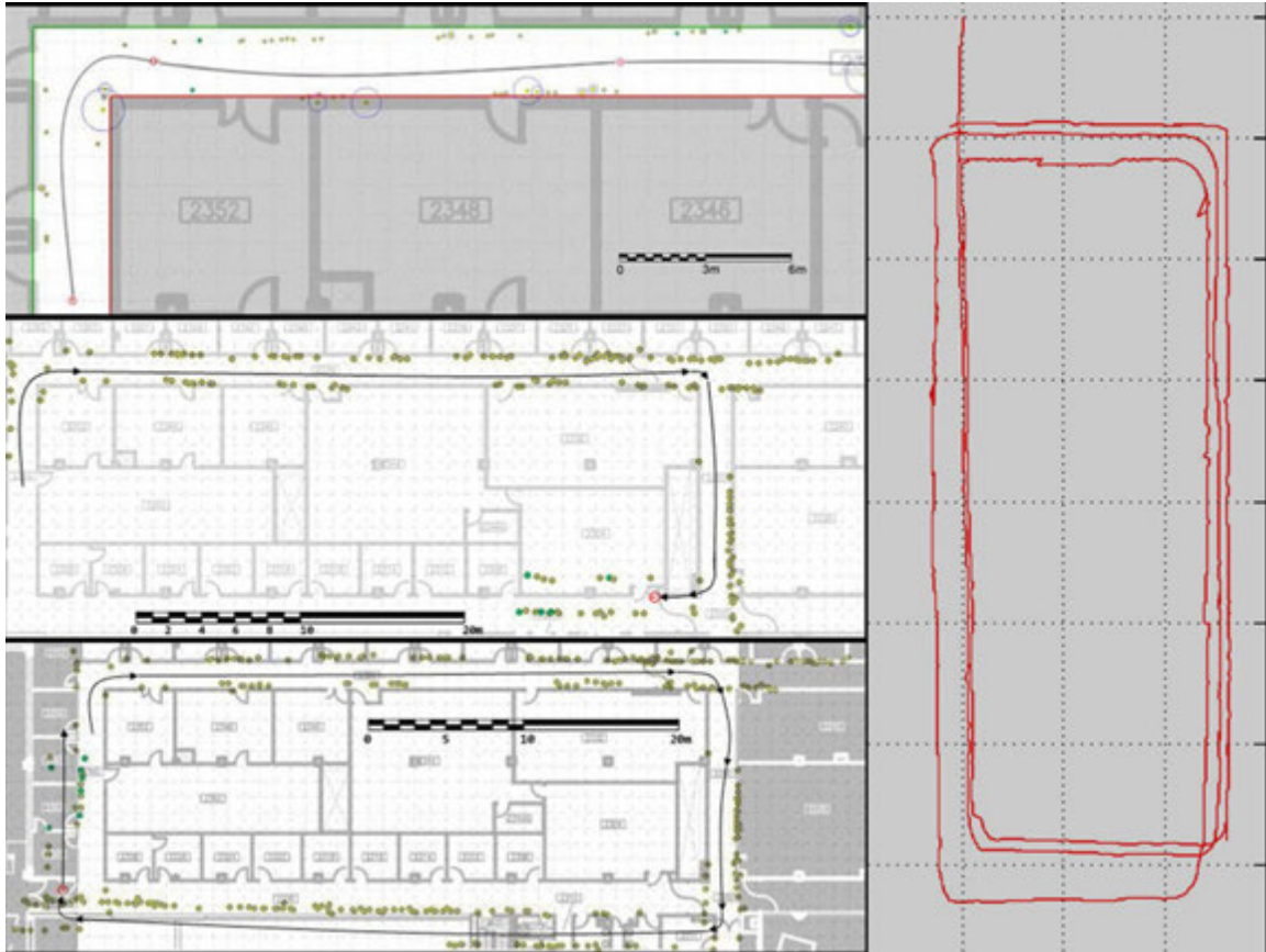
Figure 2.50: Early loop closure performance of VINAR where positioning error was reduced to 1.5 meters for a travel distance of 120 meters. In later versions the loop closure error was further reduced with the introduction of better landmark association algorithms.
