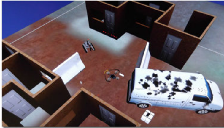
Figure 8.21: Cooperative belief of two robots, showing objects of interest for the robots as seen by their respective monocular cameras.
