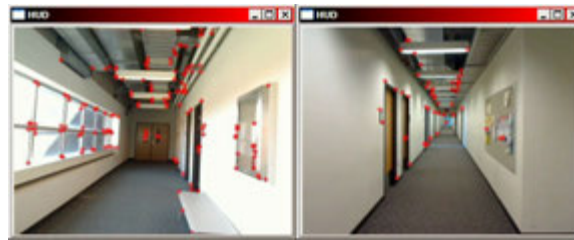
Figure 3.36: Entropy response of the landmark task. Note how the landmarks are attracted to areas with higher entropy. Uniform surfaces, such as walls, do not attract landmarks.
