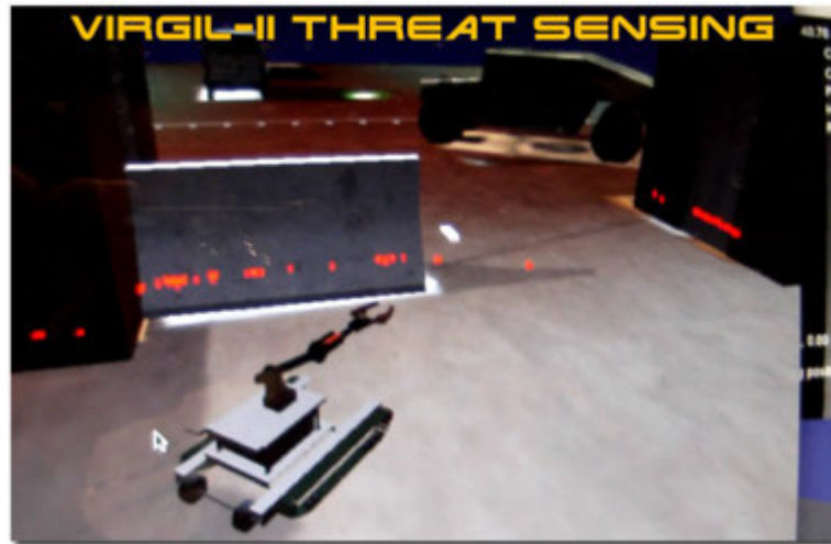
Figure 8.18: Red dots indicate range and bearing measurements Virgil is taking via VINAR. Each of these have potential to become a landmark and help Virgil map the environment.
