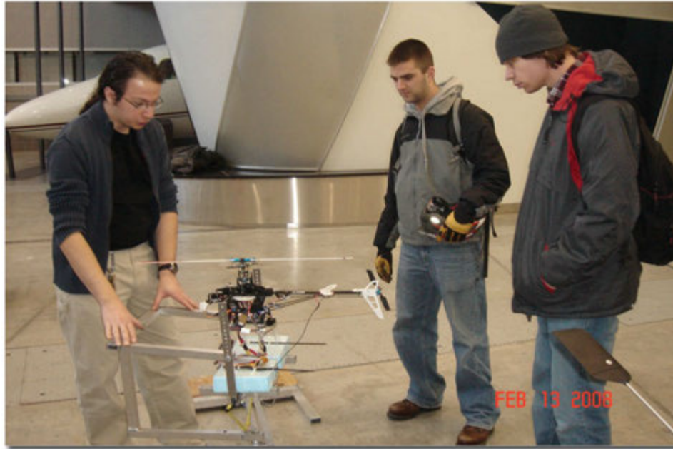
Figure 3.5: Torsional pendulum tests of Saint Vertigo V2.0 to determine moments of inertia around the fuselage around center of gravity. Blades rotate clockwise, in contrast to most full-size helicopters. The direction does not have an effect on aircraft performance. Clockwise rotation was selected because counter-clockwise one-way bearings at this small scale were not available at the time, and cost of manufacturing one did not justify the gains.
