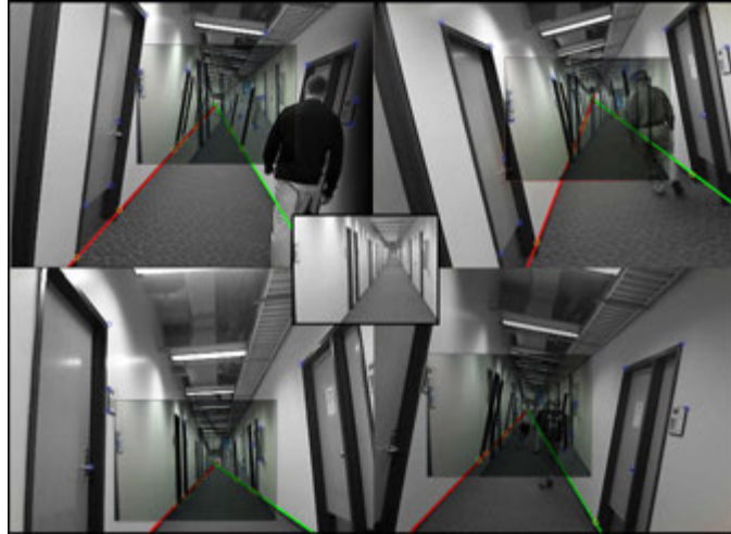
Figure 2.53: Data association metric used in Saint Vertigo where a descriptor is shown on the middle.
