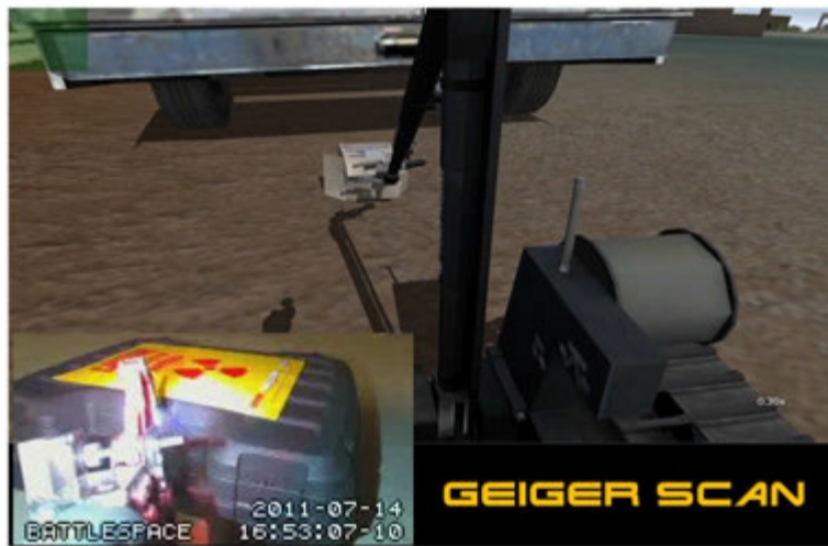
Figure 8.12: Virgil, inspecting an alpha emitter based mock IED - both real and virtual environments are shown. The bag contains a small ore of Americium which attracts the Geiger counter on the robot, and VINAR is used to navigate to the bag.
