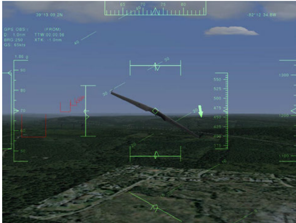
Figure 7.36: MINA Flight Simulator rendered in chase-view. A single patch of scenery from aerial images is shown opposed to tile-generated scenery. Chase-view is there to help a human pilot control the aircraft for custom flights, the HUD serves the same purpose. These are not needed for the autopilot system and not rendered on output frames.
