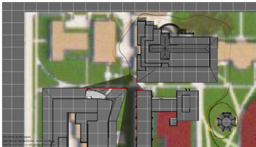
Figure 6.27: State observer during Example-3. Yellow path represents belief, black path represents ground truth.
