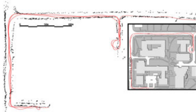
Figure 2.58: Results of the proposed ranging and SLAM algorithm from an outdoor experiment in an urban area. A small map of the area is provided for reference purposes (not provided to the algorithm) and it indicates the robot path. All measurements are in meters. The experiment was conducted under sunlight ambient conditions and dry weather.
