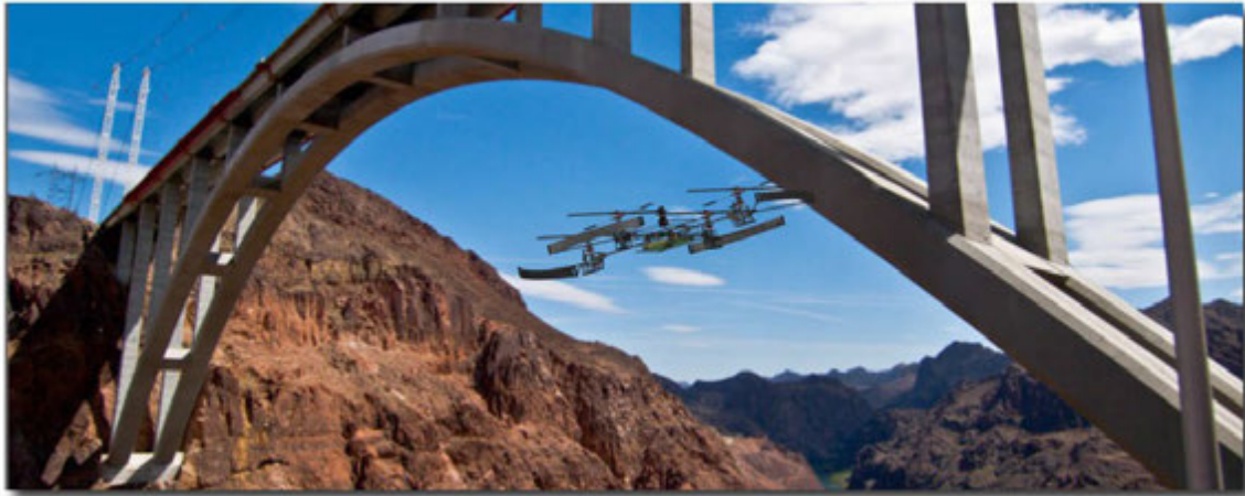
Figure 3.49: Illustration of Dante airborne sensor platform inspecting the Hoover Dam Bridge.
