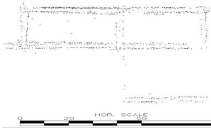
Figure 2.55: Experimental results of the proposed ranging and SLAM algorithm; showing the landmarks added to the map, representing the structure of the environment. All measurements are in meters. The experiment was conducted under incandescent ambient lightning.
