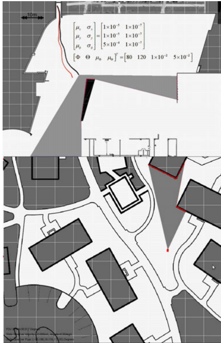
Figure 6.13: State observer interacting with the world, both floor-plan and BEV maps are displayed.
