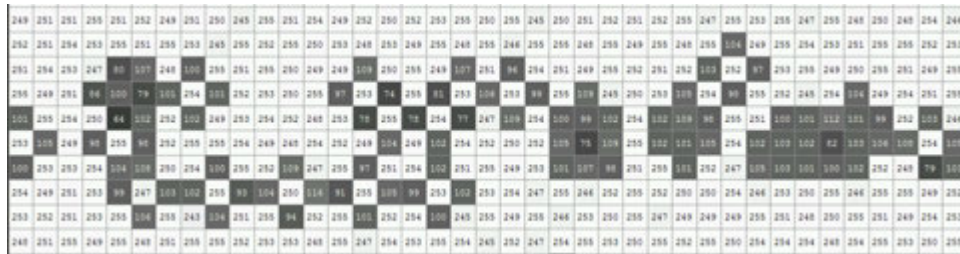
Figure 4.25: This figure shows a flat wall in an occupancy grid map at 1600× magnification where individual pixels are visible. Darker colors indicate obstacles. The dents in the wall are indeed sensor noise, which make the wall look like it was riddled with bullets at this level of magnification, which is not true.
