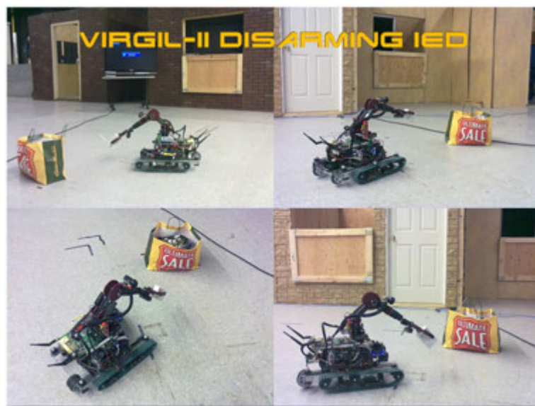
Figure 8.20: Virgil placing a remote controlled detonator inside a suspicious package. In order for the mission to succeed the robot must recognize the foreign object in the map, find it, and place detonator without triggering any charges.
