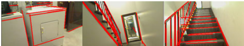
Figure 5.47: T6-Lens detecting lines and points. Points can be tracked more robustly than lines, even in distortion. For that reason points that naturally reside on lines are particularly useful because they can be used to form a Radon Snake.
