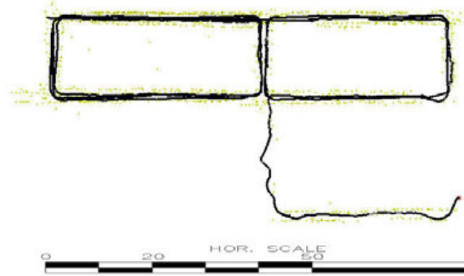
Figure 2.56: Top: Experimental results of the proposed ranging and SLAM algorithm with state observer odometer trail. Actual floor-plan of the building is superimposed later on a mature map to illustrate the accuracy of our method. Note that the floor-plan was not provided to the system a-priori. Bottom: The same environment mapped by a ground robot with a different starting point, to illustrate that our algorithm is compatible with different platforms.
