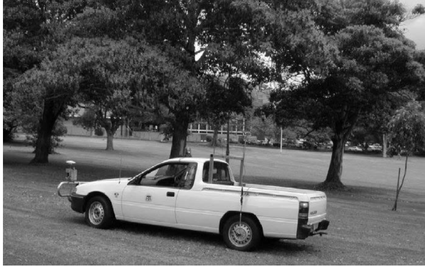
Figure 4.16: CEKF Vehicle in Victoria Park. Note the scanning laser range-finder mounted on the front bumper - this is the main sensor for the vehicle with a 180 to 240° FOV depending on the model.
