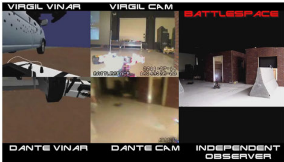
Figure 8.15: Live screenshot of Virgil-Dante cooperation while the robots team up to find and disable an IED. There are three cameras; one on each robot and an independent observer, not connected to any of the systems but there for reporting purpose only. For each robot camera, there is a virtual camera representing the robot belief of 3D objects around.
