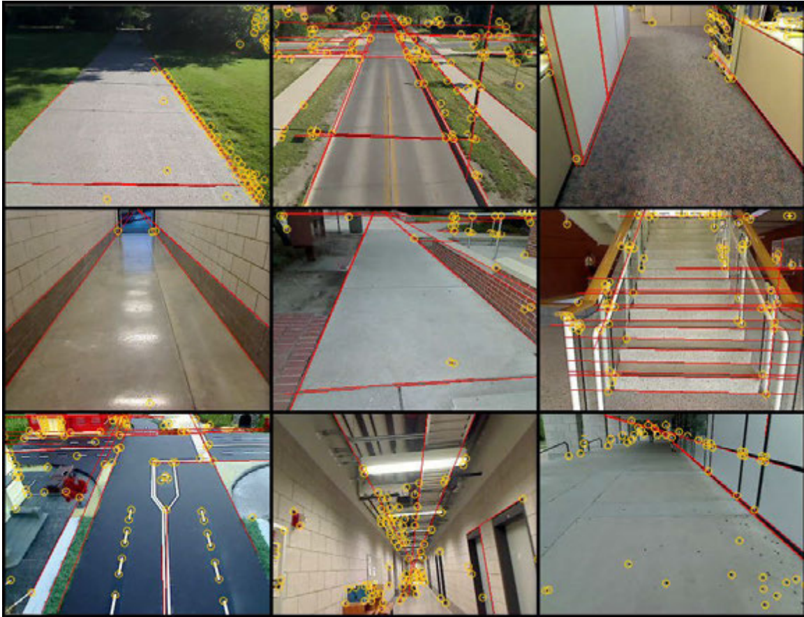
Figure 2.34: While this thesis emphasizes hallway like indoor environments, our range measurement strategy is compatible with a variety of other environments, including outdoors, office environments, ceilings, sidewalks, building sides, where orthogonality in architecture is present. A minimum of one perspective line and one feature intersection is sufficient.
