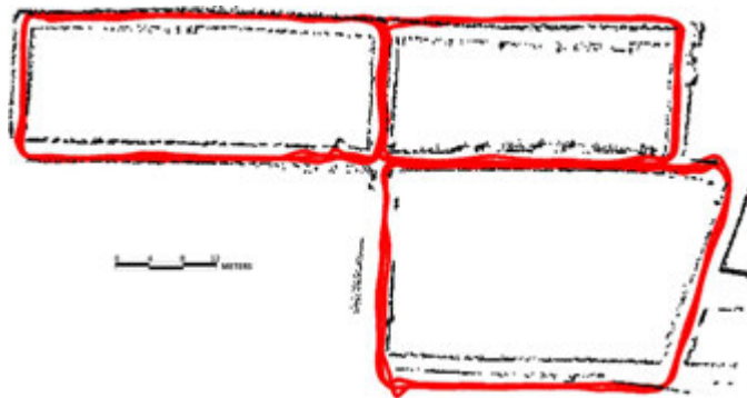
Figure 2.57: Results of the proposed ranging and SLAM algorithm from a different experiment, with state observer ground truth. All measurements are in meters. The experiment was conducted under fluorescent ambient lighting, and sunlight where applicable.
