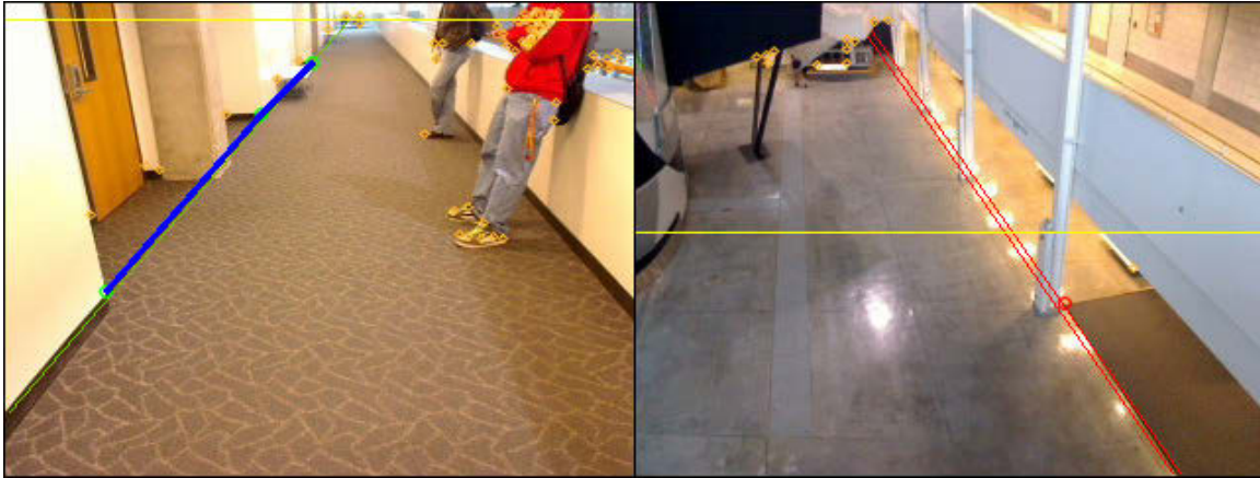
Figure 2.30: The final stage of extracting hallway lines in which segments are being analyzed for collinearity. Note that detection of two lines is preferred and sufficient, but not necessary. The system will operate with one to four hallway lines.
