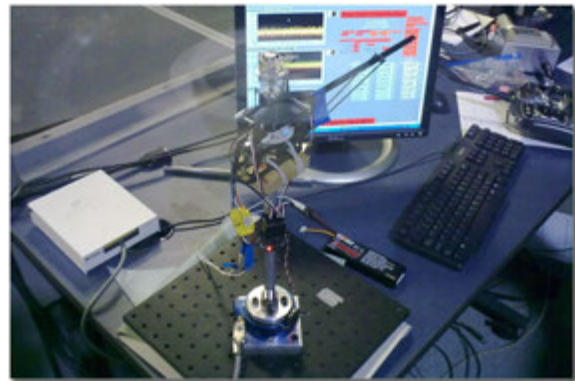
Figure 3.4: Long hours of wind-tunnel testing had to be performed on Saint Vertigo to determine the optimal rotorhead and powerplant combinations. After experimenting with several different rotor designs, phasing angles, and multi-blade systems, wind-tunnel data gathered during the conception stage indicated the optimal lift ratio is achieved with two blades and even then aircraft flies with heavy wing loading. Propulsive efficiency is poor at this scale airfoils because our atmosphere does not scale with the aircraft. Induced drag from increasing the number of blades did not bring justifiable gains in flight performance, so two bladed design was kept.
